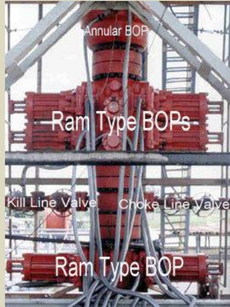
BOP Stack with multiple rams
